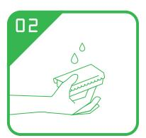
Wrap the microfiber suede around the applicator block. Carefully open the bottle and apply one ot two lines of HYPER BOROPHENE COATING onto the applicator.
