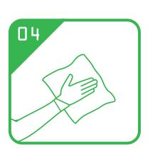
The ideal flashing time is 2-4 minutes at a temperature of 24 °C. If the temperature is lower, wait longer. Once it feels slightly tacky, gently wipe it off with a microfiber towel, being careful not to apply too much pressure.
